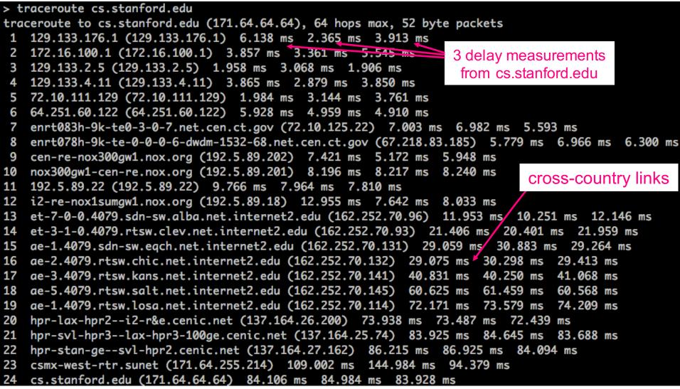
\* means no response (probe lost, router not replying)
