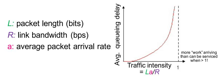
*La*/*R* ~ 0: small avg. queueing delay *La*/*R* $\rightarrow$ 1: large avg. queueing delay *La*/*R* > 1: infinite avg. queueing delay
