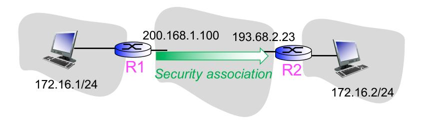
R1 sends IPsec pkt: R1 accesses SAD to determine how to process R2 gets IPsec pkt: R2 uses SPI into index SAD, processes pkt accordingly
