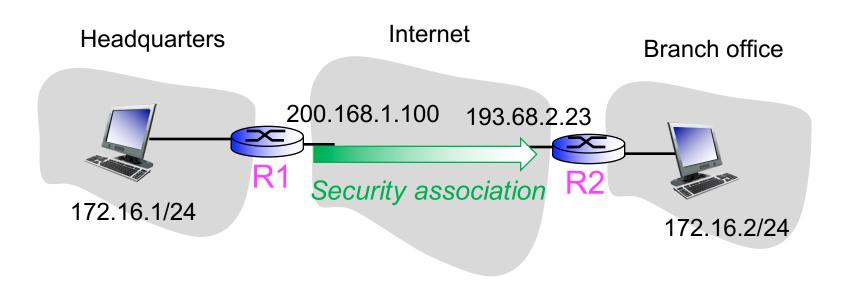
2. Encrypts result using algorithm & key specified by SA
